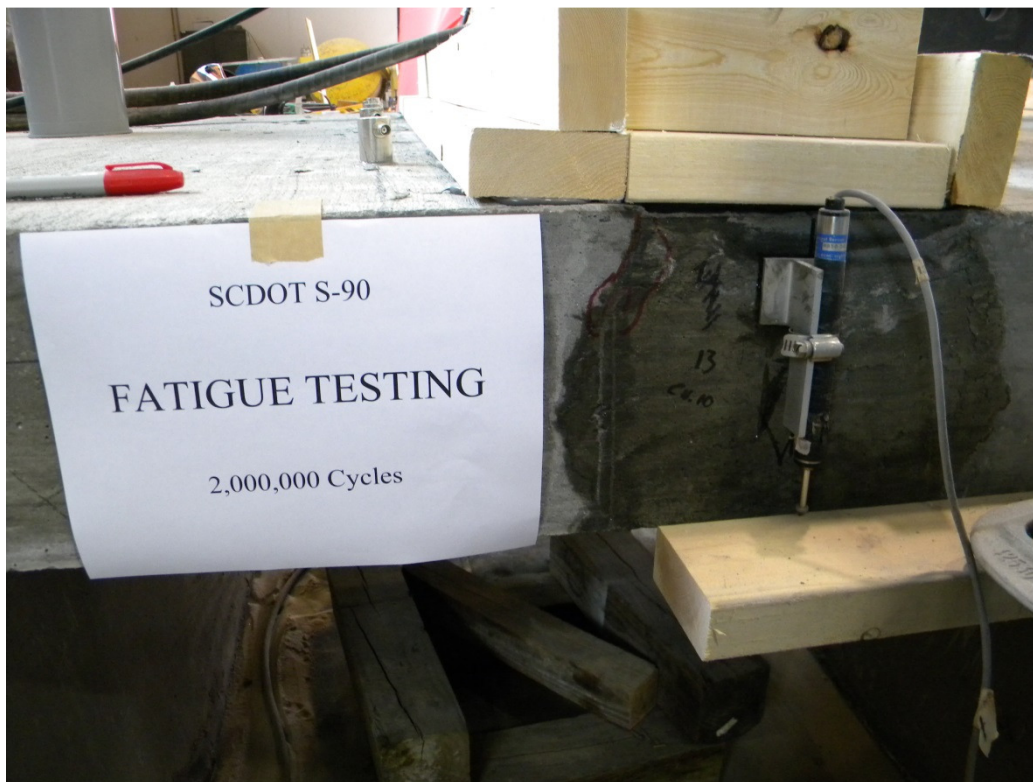
Figure 3.22: Joint condition following fatigue testing
