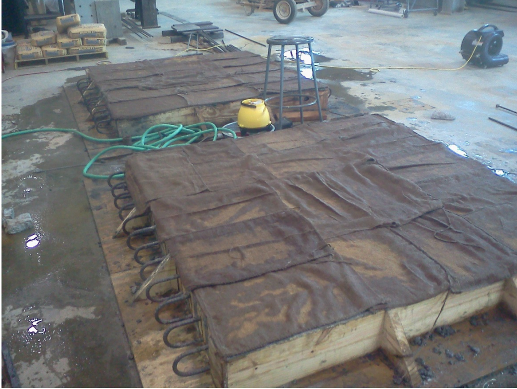
Figure 3.9: Specimens being moist cured
