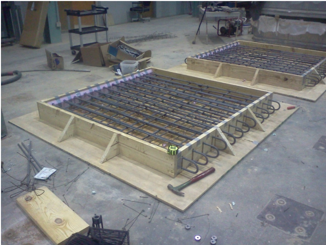
Figure 3.8: View of both specimens with rebar
