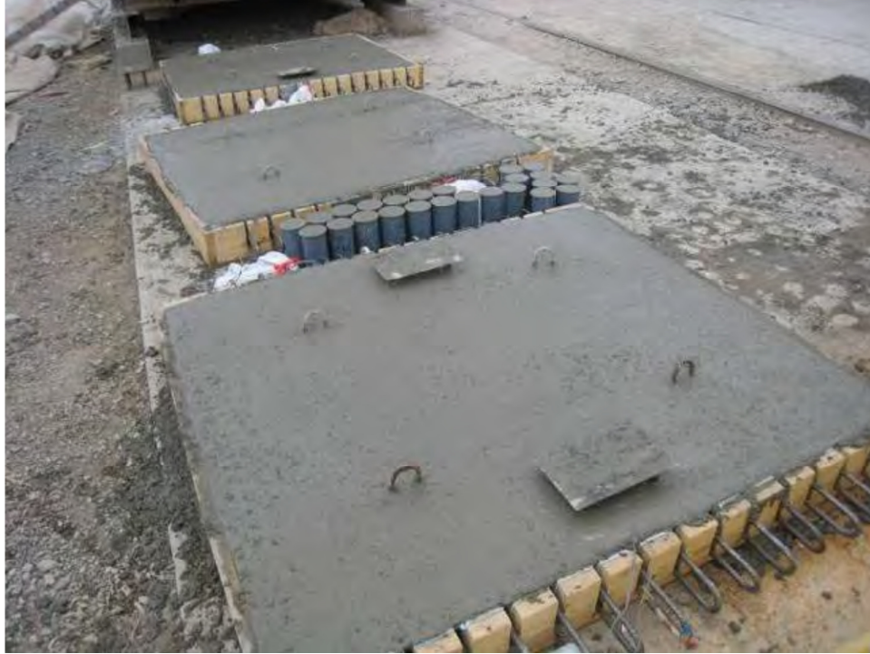
Figure 2.6: Large scale specimens after pour (French, et al., 2011)
