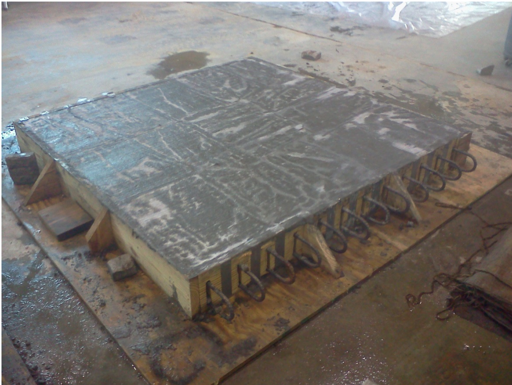
Figure 3.9: Specimens being moist cured
